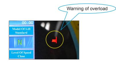
Forbid lift with load over 10% of the standard
