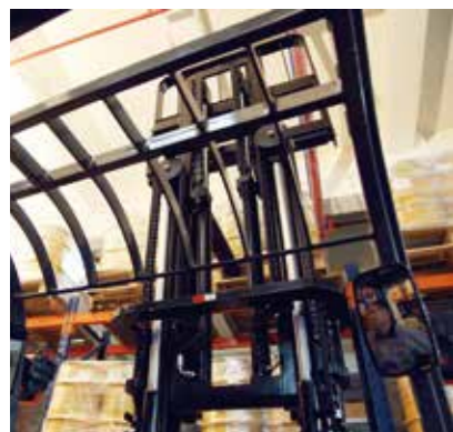
Triplex mast with dual free lift cylinders
