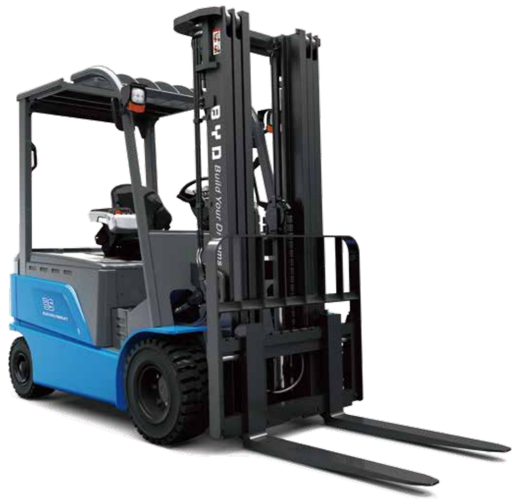
Comfort equipment: full suspension seat, fingertip controls, triplex mast with dual free lift cylinders, and 4 way hydraulic valve.
